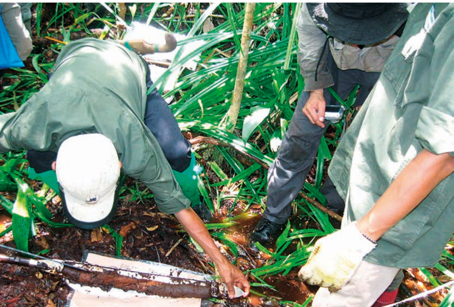
Measurements are taken for carbon assessment in peat swamp forests in Central Kalimantan, Indonesia, during the REDD+ Feasibility Study 2012. Photo: FORDA
