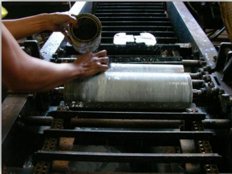
Photo 46 (by Kim): cleaned glue spreader economize glue consumption (46)
