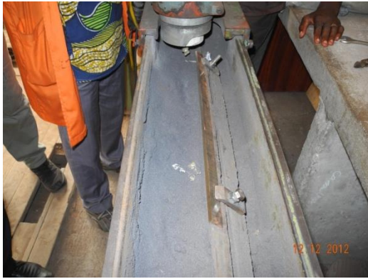
Photo 65 (by Kim): knife grinding without coolant (65)
