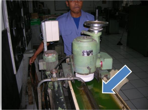
Photo 66 (by Kim): knife grinding with coolant (66)
