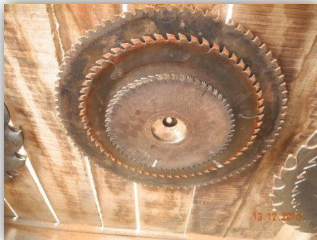
Photos 67-68 (by Kim): improper storage of saws: circular saws lumped together (67) and band saw blade rolled and kept on the floor (68)
