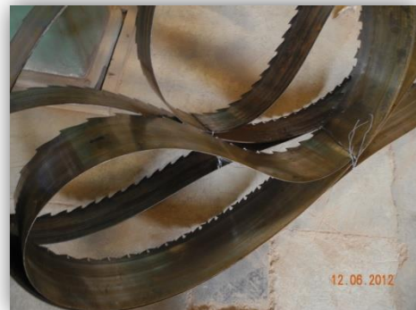
Photos 67-68 (by Kim): improper storage of saws: circular saws lumped together (67) and band saw blade rolled and kept on the floor (68)
