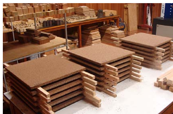
The end-product: Particleboards produced from the wood waste of various species. Photo: Paula Gabriella Surdi
