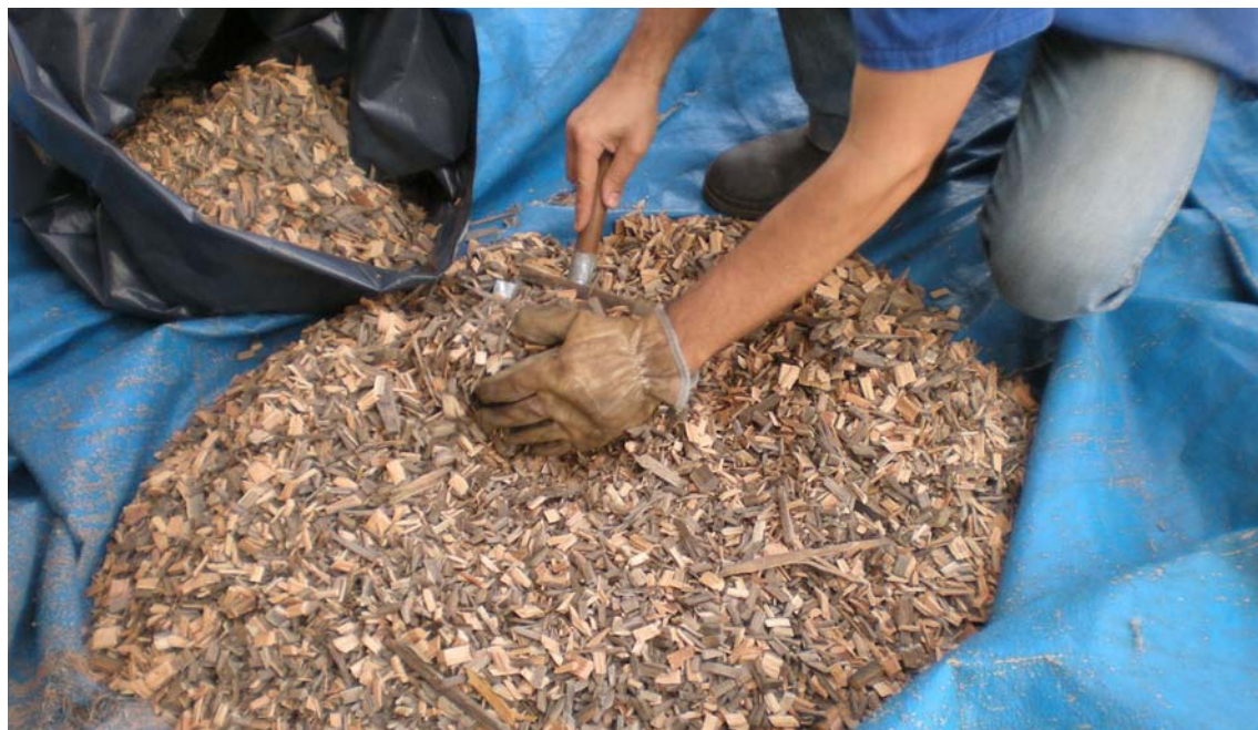
Leftovers: Sawmill residues were transformed into chips to produce particleboard. Photo: National Hardwood Flooring Association
