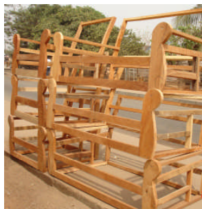
Poorly assembled frames made of any species
