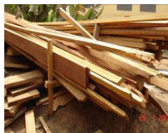
Poorly stacked wood with high MC and low grade for furniture
