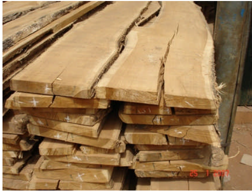
92% of this lumber had splits and other defects
