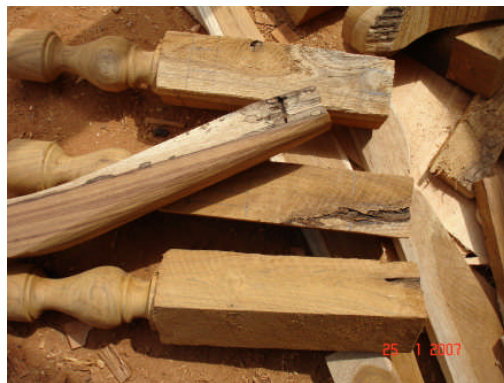
Highly defective wood moulded as furniture legs
